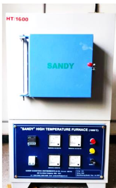
Muffle Furnace (Sandy Scientific, Chennai) up to 1500°C
