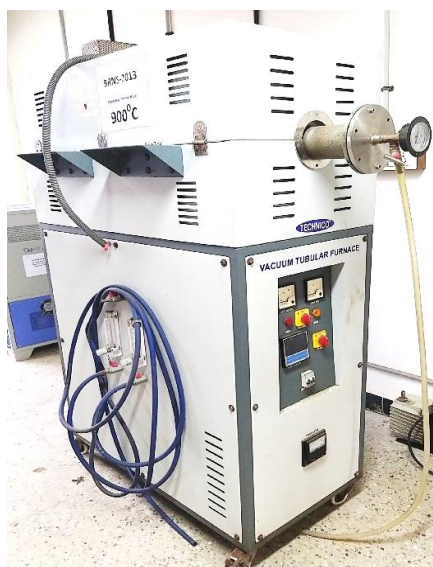
Tubular Furnace (Technico, Chennai) up to 1000°C
