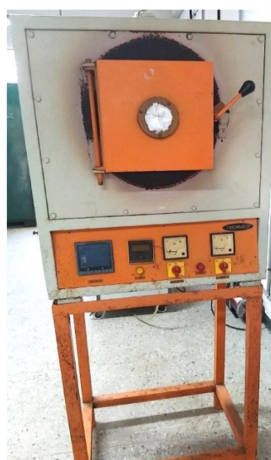
Muffle Furnace (Technico, Chennai) up to 1200°C
