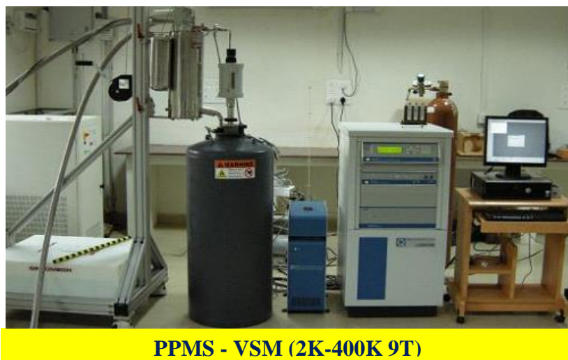
Figure 17. Photograph of a Physical Property Measurement System - Vibrating Sample Magnetometer (Quantum Design, USA) setup.
